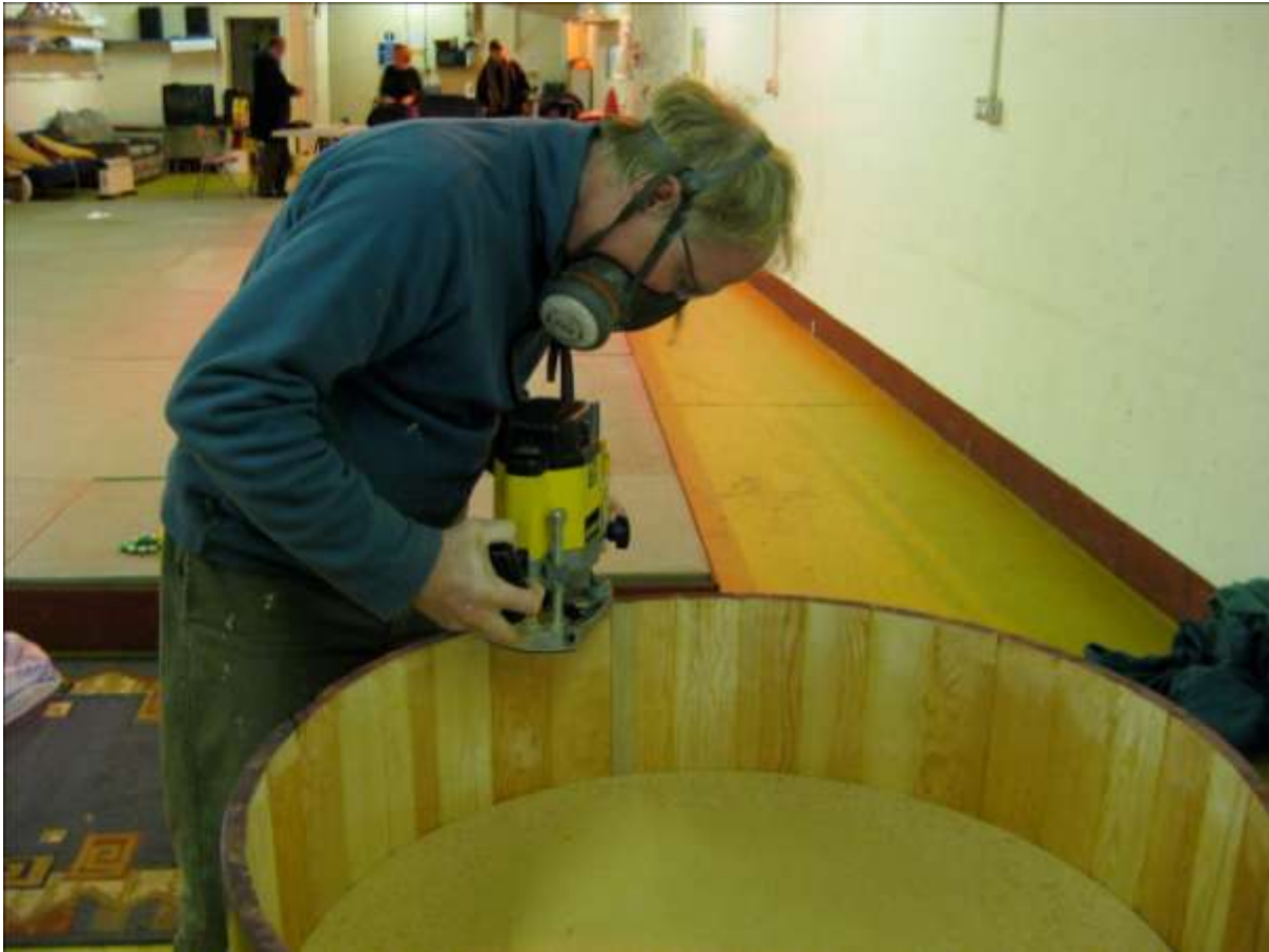
Andrew making the bearing edge with a router.
